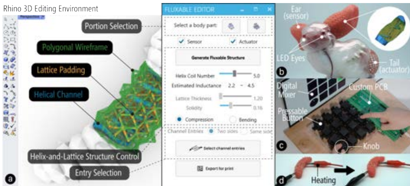
Figure 1: 3D printable sensors and actuators are created with (a) Fluxable design tool, such as (b) a Pomodoro bunny timer, (c) a DJ BeatPad, and (d) a caterpillar robot.
