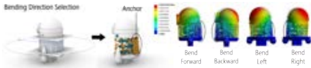
Figure 2: Lattice with higher density can be added to the lattice padding as ‘anchors’ to achieve desired lateral bending behaviors: the Finite Element Analysis (FEA) showcases four directional bending examples.
