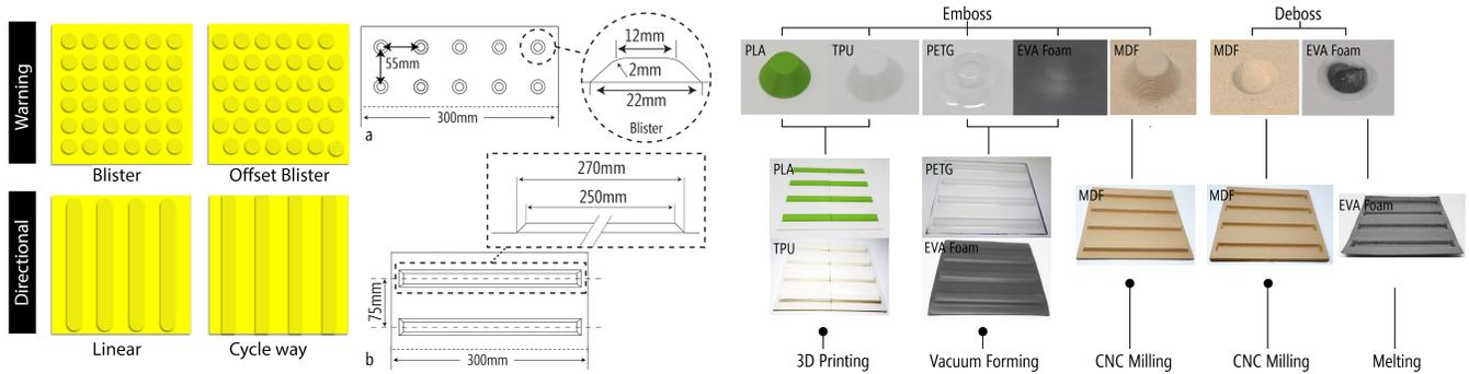
**Figure 2: The standard tactile surface indicator designs for the warning (truncated domes) and directional guides (rectangular bars). Diagram showing the dimensions and spacing of the bars and blister designs (middle). Detailed prototypes (left to right): 3D printing, vacuum forming, CNC milling, and melting and varied design elements—embossed and debossed features (right).**
