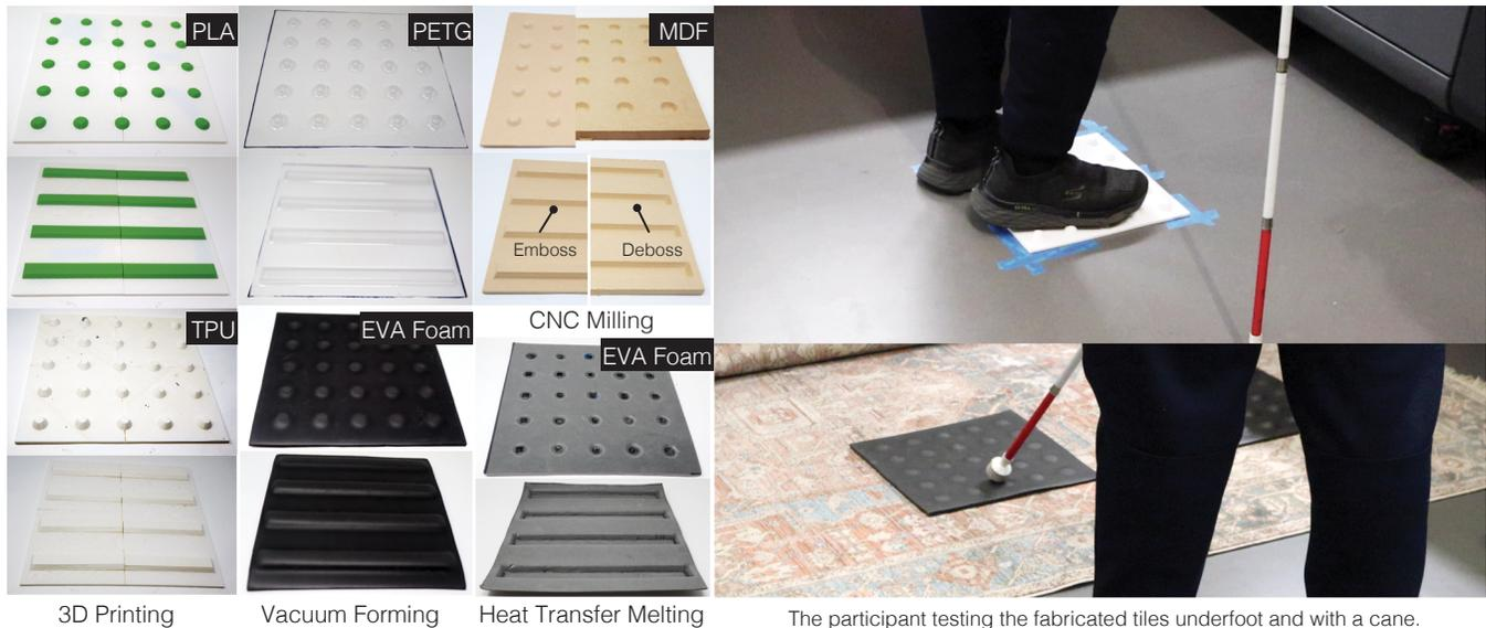
**Figure 1:** Samples of tactile surface indicators (TSIs) created via rapid prototyping methods (left) such as 3D printing, vacuum forming, CNC milling, and heat transfer melting—(right) which were evaluated through a qualitative study with a blind cane user to validate their tactile saliency as well as an O&M specialist.
